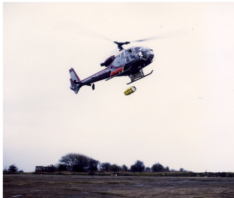
SAFKEG undergoes a drop test
