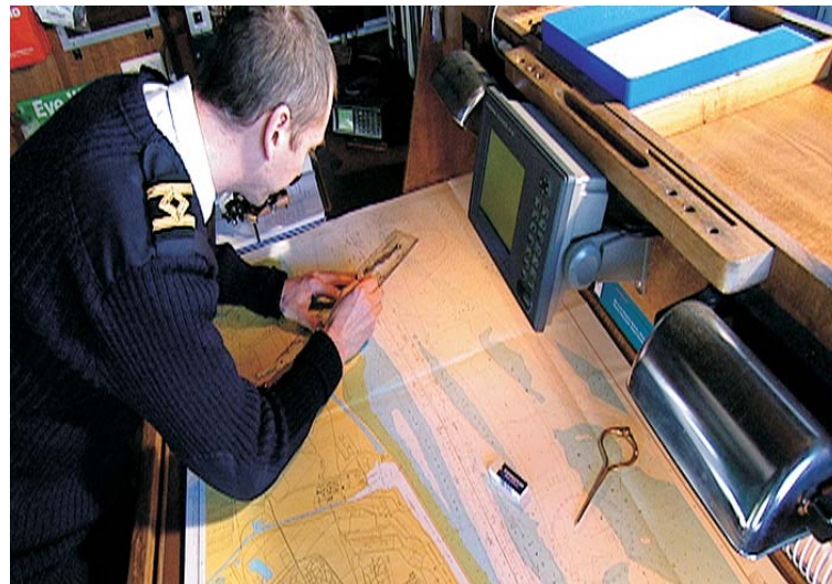
Manually plotting courses is one of several backup navigational systems on the Atlantic Osprey
